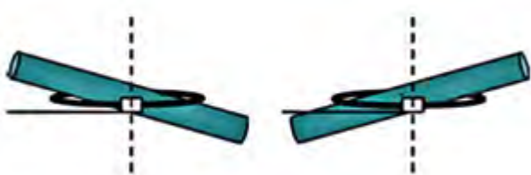
Figure 7: Orthogonality effect. Primary conductor position versus the axis of the Rogowski loop.
